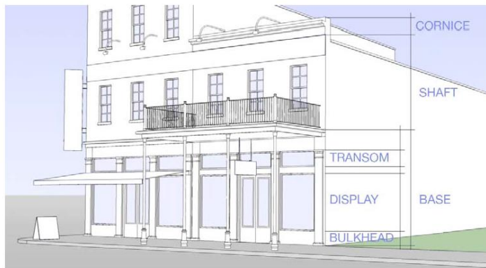
Figure A- 1 Shopfront Elevation Elements
