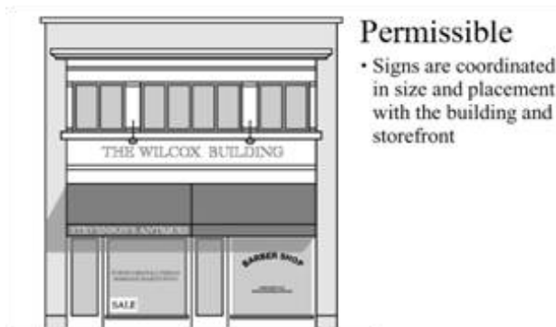
Figure 64-13-7.1 Permissible Signage Placement
