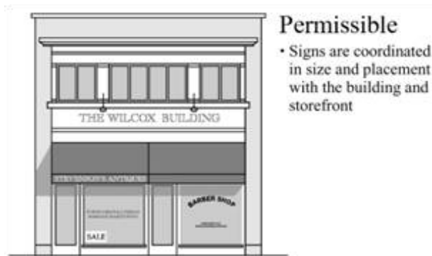
Figure 64-13-7.1 Permissible Signage Placement
