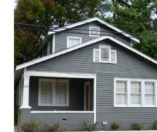
Place an addition so that it is subordinate to the historic residential structure by having a break in the wall plane, and stepping back the addition from the primary facade.
